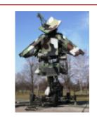
One reconditioned SNR-125 Mobile Radar Station. This unit is able to search out to 15 miles for air threats. It gives the defenders time to get under cover, and the air defences some warning of direction, speed and altitude of the attacker, significantly enhancing their chances of a successful engagement when the attacker arrives. It is towed by any vehicle.
