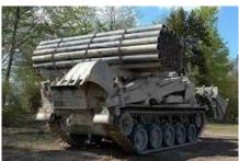
A fascene is a bundle of steel pipes that are carried into battle to fill in anti tank ditches to create a crossing point. Any Truck can carry 2, and armoured vehicles can carry 1. Once used, they are considered expended, but give your forces vital ability in crossing an Anti Tank Ditch.
